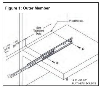
Attach the drawer to the extended inner members with the # 10 - 32 Slotted Pan Head Screw screw inserted through the vertical slots. Leave all screws loose for final adjustment. Adjust slide positions until movement is smooth. Then tighten all screws; if necessary, use more screws to secure slides and complete installation.
