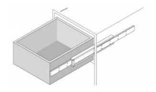
\*Note: Flat mounting is not recommended, reduces the load rating by 80%
